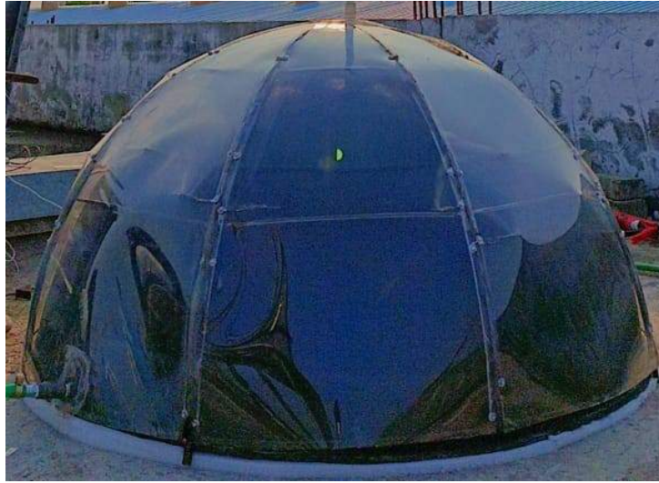
Hemispherical Solar Water Heater
