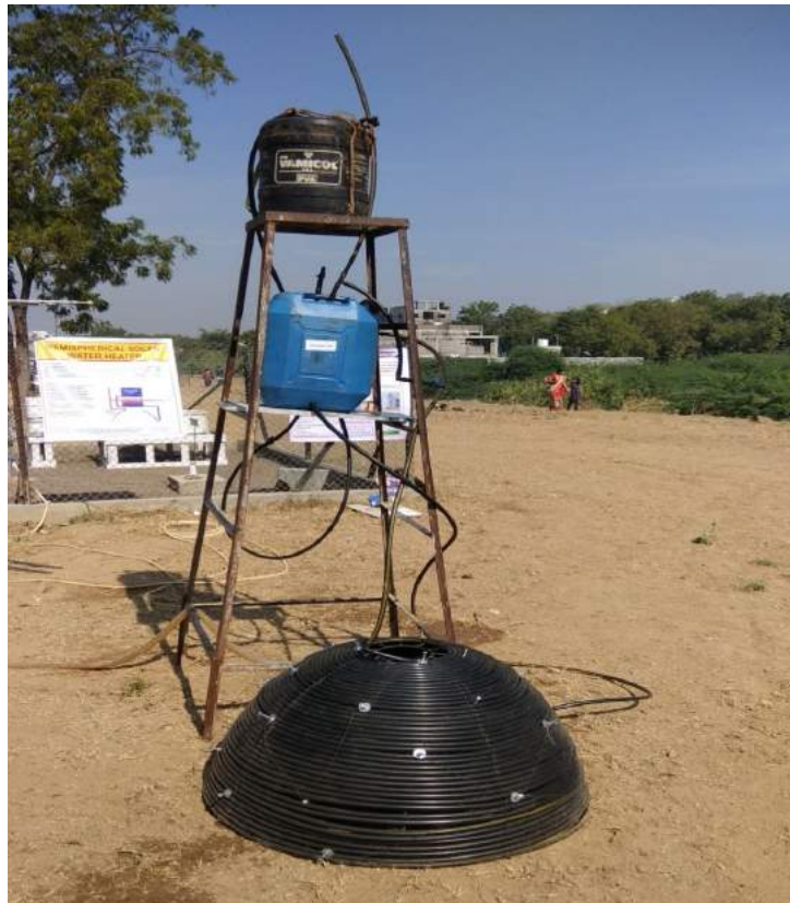
Tubular Hemispherical Solar Water Heater (75 LPD)
