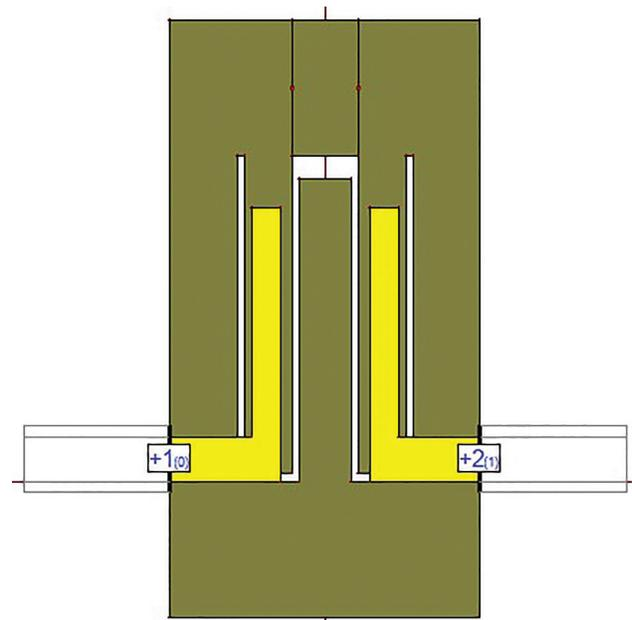
Fig. 14: UWB BPF Structure in IE3D MGRID Editor.
