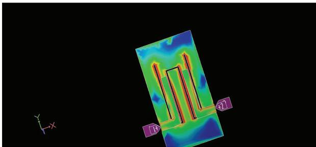
**Fig. 17: Simulation Results of Current Distribution Vs. Operating Frequency of Design 3.**
