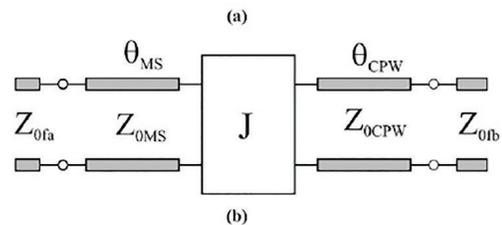
**Fig. 9: MMR on Coplanar Waveguide Transition (a) Design. (b) Corresponding Network.**
