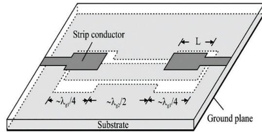
**Fig. 8: Schematic of UWB BPF (Design 2).**
