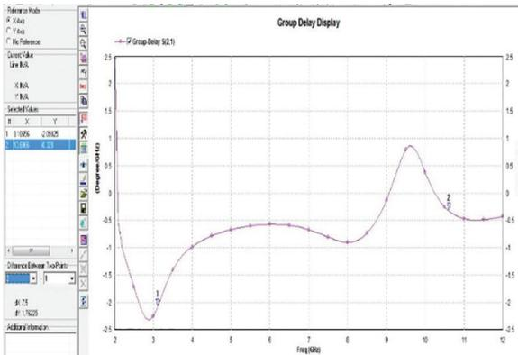
**Fig. 7: Simulation Results of Group Delay Vs. Operating Frequency of Design 1.**
