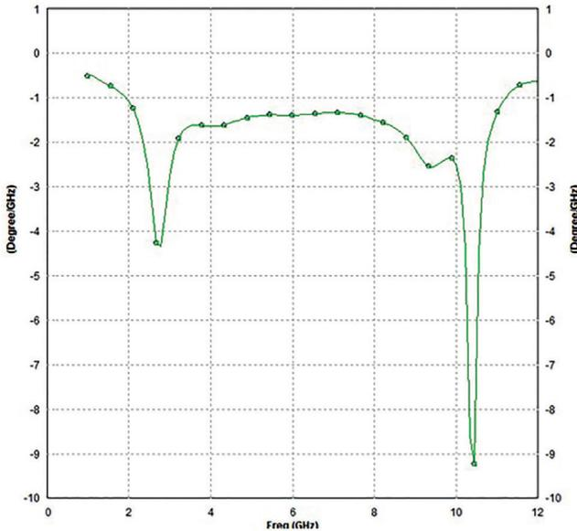
**Fig. 16: Simulation Results of Group Delay Vs. Operating Frequency of Design 3.**
