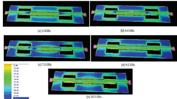
**Fig. 12: Simulation Results of Current Distribution Vs. Operating Frequency of Design 2.**
