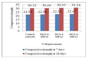
Fig 1- Compressive strength Vs Mix -I
