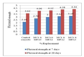
Fig 11. Flexural strength Vs Mix –III
