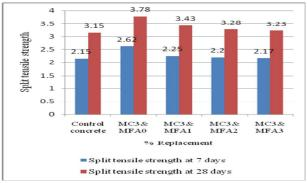
Fig 8 Split tensile strength Vs Mix – IV
