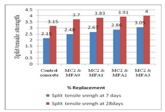
Fig 7 Split tensile strength Vs Mix III
