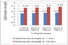
Fig -5 Split tensile strength Vs Mix -I
