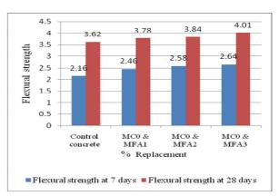
Fig 9 Flexural strength Vs Mix -I
