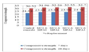
Fig -3 Compressive strength Vs Mix- III
