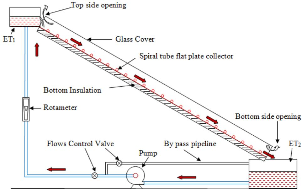
The convective heat loss coefficient from the top surface of glazing to the atmosphere is given by Tiwari (2013),  $h_{c_2} = 2.8 + 3.0 W$ , where  $W$  is the wind velocity over the top glass cover.
