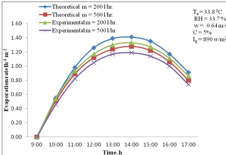
Figure 4 Effect of concentration on evaporation rate (see online version for colours)
